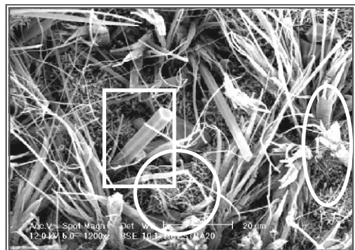
Fig. 3. Aluminum, boron and mixed oxides, sintering at 1373 K for 30 min.
