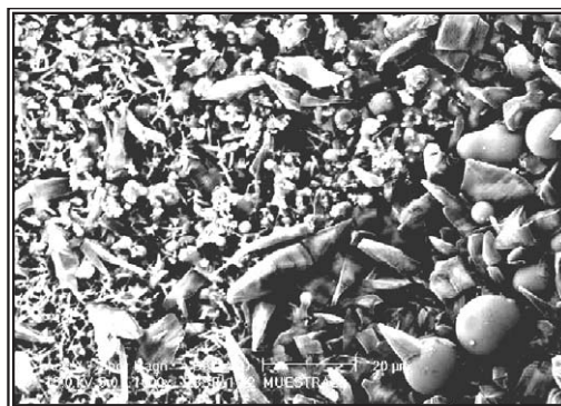
Fig. 4. Aluminum oxides, sintering at 1373 K for 30 min.
